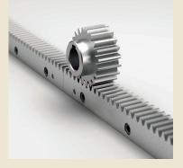
A rack and pinion comprises a circular gear (the pinion) engaging a linear gear (the rack). Together, they convert rotational motion into linear motion. Rotating the pinion causes the rack to be driven in a line. Conversely, moving the rack linearly will cause the pinion to rotate.
