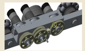
When you are meshing gears, you have to be sure that the gears are not too loose nor too tight. If the gears are too loose, the teeth will easily wear out, decreasing its longevity. But if they are too tight, they will have too much friction and possibly grind or bind up. **The ideal way to mesh gears is to make sure the teeth interlock and just touch the base of the gear.**
