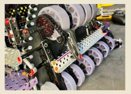
These intakes work by having a hard or pliable object rotate along an axis. For this it can be used different types of wheels (compliant, solid traction, foam wheels) in order to propel the game element to the storage or directly to your out take.
