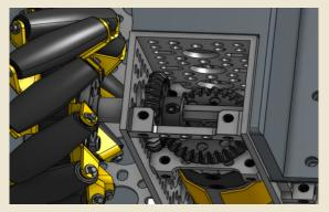
Miter gears are bevel gears which have a 1:1 ratio between the drive gear and driven gear. They are used especially for drivetrains. Their steel construction and large tooth size make them perfect for high-torque applications.
