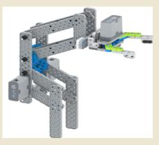
It is an extension of the four bar linkage because at the end of the four bar is mounted another one. This requires large space, but is a compact method of making large amounts of linear extension.
