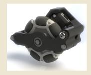
Dead wheels typically consist of 2 or 3 unpowered omni wheels mounted on a robot, with at least one of them oriented perpendicularly to the others. These wheels should be positioned along the circumference of a circle inscribed on the robot. To ensure optimal performance, dead wheels require a reliable **counterspring**, which can be created using a spring or surgical tubing. The use of countersprings makes odometry pods more precise than the encoders on your motors. For instance, if
