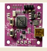
An Interial Measurement Unit (IMU) is a combination of a Gyroscope, Accelerometer, and Magnetometer. A Gyroscope is a device that reports the angular orientation of an object in 3 dimensions. An Accelerometer is a device that reports the acceleration of an object in 3 dimensions.
