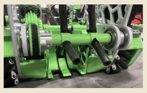
A direct transfer is the mechanism in which the items are moved to. It is placed behind whatever is picking up the game elements. It usually consists in an arm or a bucket to collect the items as soon as they enter the intake.
