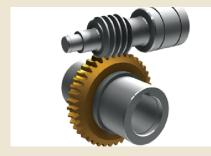
A worm drive is a gear arrangement that uses a worm (a gear in the form of a screw) and a worm wheel (which is similar in appearance to a spur gear). The two elements are also called the worm screw and worm gear. Worm drives are a compact means of substantially decreasing speed and increasing torque.
