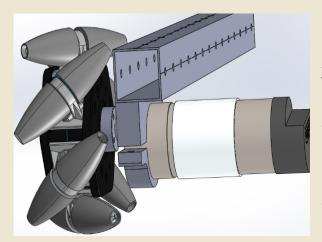
drive Direct consists in powering а mechanism directly from the motor axis. This way you put unnecessary load on the drive motor. This is because the shock loads can destrov gearboxes. Gearboxes are able to resist load along the axis of rotation for example when the wheel changes direction. However, in direct drive the gearbox shaft can be exposed to other shock loads outside of the normal axis for example when the wheel comes into contact with another robot.
